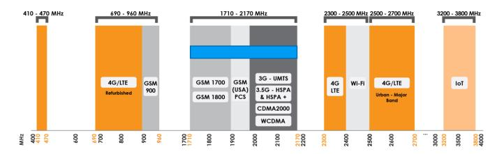
Indicates the LTE bands on which HELI-5 works
