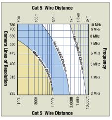
All measured distances include any coax in the path. Wire resistance may be measured with an ohm-meter by shorting the two conductors together at the far end, and measuring the loop-resistance out and back.
