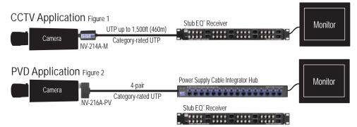
The StubEQ<sup>TM</sup> Receiver Hub is an active (amplified) hub that allows the transmission of real-time monochrome or color video for distances up to 1,500ft (460m), (2,000ft (600m) if the transmitter is a NV-653T). using Category-2 or better Unshielded Twisted-Pair (UTP) wire. The receiver hub continuously and automatically compensates for cable attenuation, and ground-loops, independent of the video signal image. The 1U high hub is equipped with multi-stage transient protection.
