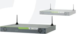
**SIM Racks** provide central SIM cards storage and eliminate the need to physically store the cards in the GSM/3G Gateways.
